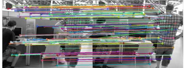
(a) Feature matching between reference frame and current frame before GC-RANSAC
