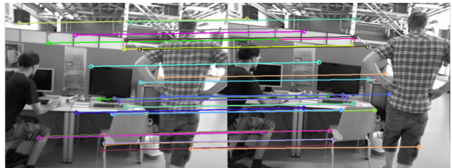
(b) Feature point pairs labeled as inliers after GC-RANSAC
